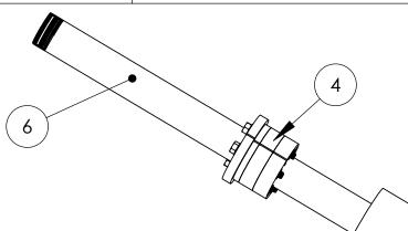
This setup is used for all Hydrant Brands using a 1-1/4" Pipe with 1" NPT Female end.
